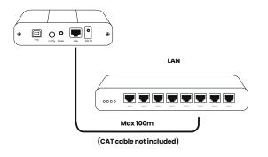
Place the Remote Extender where desired. Connect a CAT 5e/6/7 patch cable to the RJ45 Link port on the Remote Extender to an IEEE 802.3at - PoE+ (25.5W)
