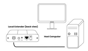
Connect a CAT 5e/6/7 patch cable from the RJ45 Link port on the Local Extender to an IEEE 802.3at - PoE+ (25.5W) capable LAN port.
